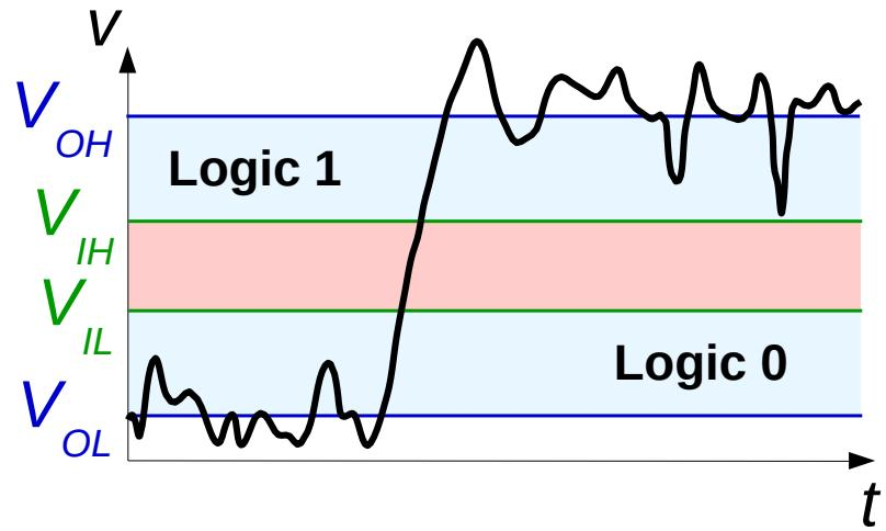
Why we still use it? Because after passing through an IC or a gate inside an IC - the signal is "rebuilt" and if the "digital discipline" described in the following is respected - we can preserve the information after numerous "passes". Thus, each element can behave with a large margin for error, yet the final result is correct.
