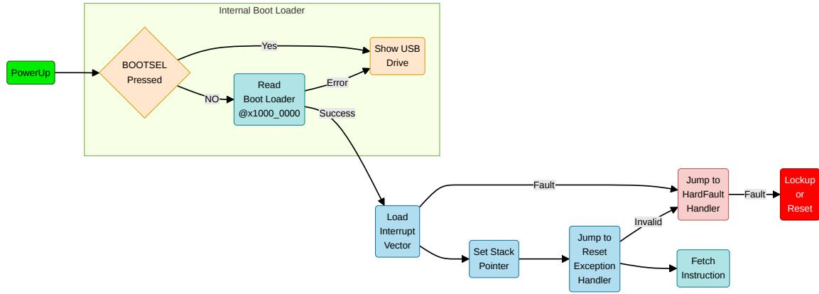
The internal boot loader cannot be overwritten and assures that bricking the device is difficult.
